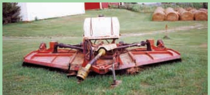
Jack Delaney strapped a 100-gal. spray tank to the top of his Bush Hog rotary mower.
