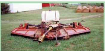
Jack Delaney strapped a 100-gal. spray tank to the top of his Bush Hog rotary mower.
