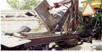
Ray Mickan's home-built tire cutter mounts on a tractor 3-pt. hitch and uses a hydraulically-powered knife to cut through tires.
