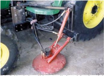
Hydraulic-driven circular saw blade mounts on side of tractor in front of rear wheel. Gengler made the saw blade himself from a 20-in. coulter.
