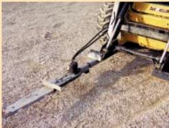
Unit's 34-in. saw bar is driven by a hydraulic motor that mounts on a short length of steel ubing. Chainsaw bar can be mounted in either a vertical or horizontal position.
