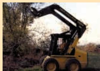
Chainsaw attachment allows Symons to cut as high as his skid steer will reach. one end of a small tube into the hydraulic line and mounting the other end to the bar post.
