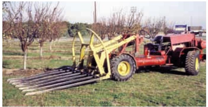
Vereschagin's brush-handling machine started out as a 1980 32-ft. diesel-powered motor home that he picked up at a wrecking yard.
