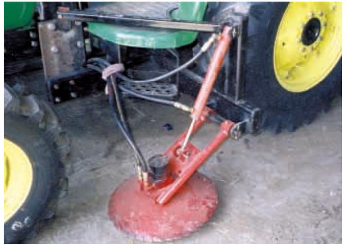
Hydraulic-driven circular saw blade mounts on side of tractor in front of rear wheel. Gengler made the saw blade himself from a 20-in. coulters.
