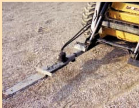
Unit's 34-in. saw bar is driven by a hydraulic motor that mounts on a short length of steel tubing. Chainsaw bar can be mounted in either a vertical or horizontal position.
