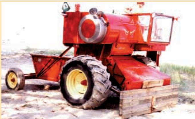
**"It makes a good dozer that I can use to push sand and even rocks," says Tom Nelson, who made a dozer blade from wood 4 by 4's and attached it to the header lift on an old combine.**
