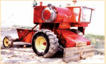
"It makes a good dozer that I can use to push sand and even rocks," says Tom Nelson, who made a dozer blade from wood 4 by 4's and attached it to the header lift on an old
