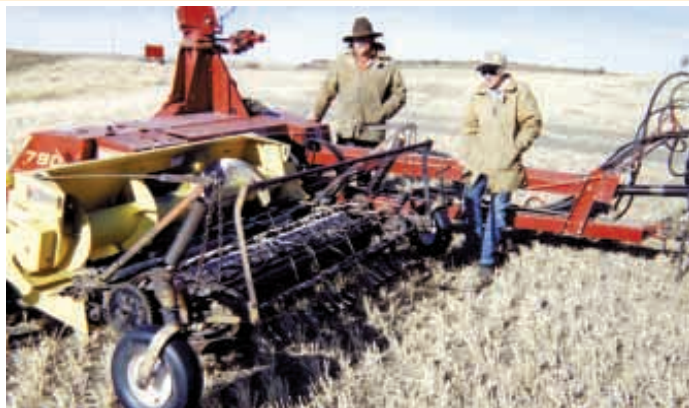
To keep rocks out of his forage harvester, Roy Klindt replaced the original pickup with a used Sund 10-ft. pickup that he cut down to match the machine.
