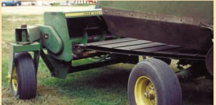
Combine's chopper drive powers a canvas conveyor that delivers straw and chaff from the sieves directly to baler throat. Chopper drive also pto-drives baler.
