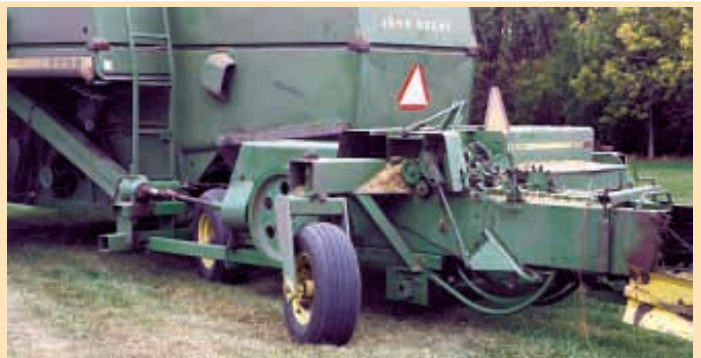
Hepfner modified a pickup from a Deere 327 small square baler so he could pull it behind his Deere 7700 combine.
