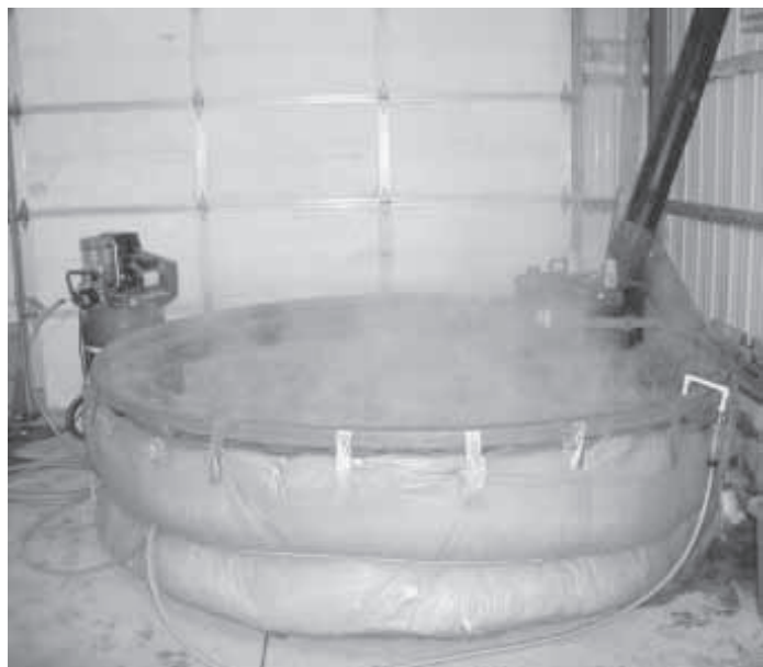
Barrel stove inside tub heats water. Hose runs from hot tub to air compressor. Note: When in use, stove is set up outside, away from noisy compressor.
