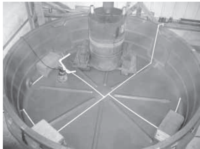
Brian Bahlmann started with a 10-ft. dia. black plastic livestock watering tank. PVC tubing at bottom of tank pumps air into water.
