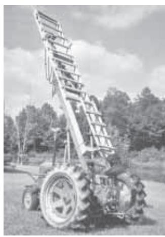
Homemade ladder is 21 ft. long when extended. It attaches to tractor's boom with U-bolts.
