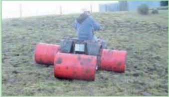
To build "The Rainy Day Roller," Paul Rivers cut the ends out of metal drums and slipped them over the wheels on his ATV.
