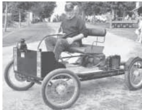
Quadricycle replica is powered by an IH 1-cyl. engine.
