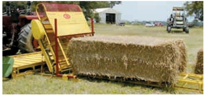
Bale feeds into separator head that pulls flakes of hay off big bale for rebaling.
