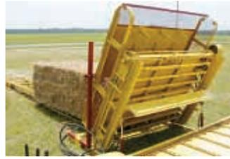
Separator head drops loose hay onto conveyor, where it feeds into small square baler.
