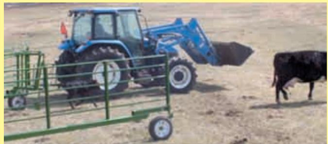
To catch a cow with tractor-pulled “cow catcher”, driver extends a cylinder to swing one side of corral out about 30 ft. away from tractor.
