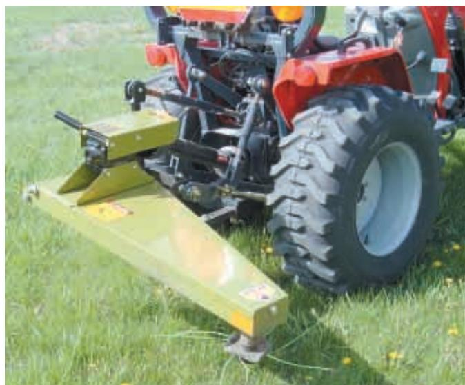
Pto-powered string trimmer can trim around and under fence lines and other hard-to-cut areas.
