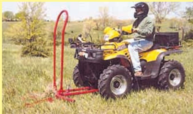
Once tree is cut, a metal guard on front forces it off to the side.
