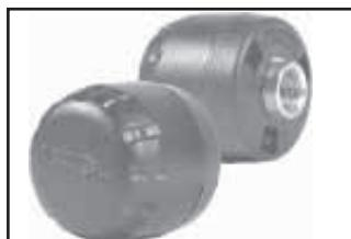
Air pressure sensors replace valve caps and send radio signals to in-cab monitor.
