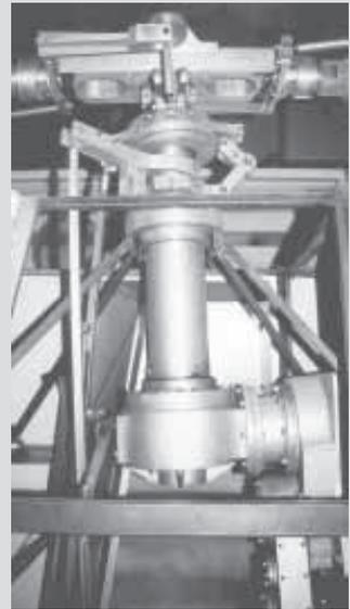
**Photo shows close-up of rotor assembly. Erickson designed and machined every part himself.**
