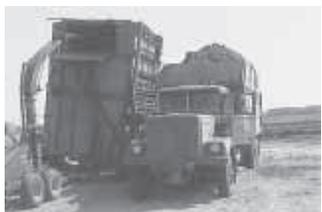
Door flips down for loading silage into wagon box.
