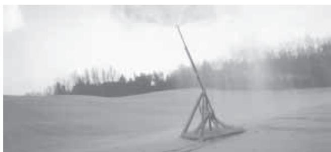
A high-pressure pump feeds well or pond water to this 22-ft. tower-type snowgun.
