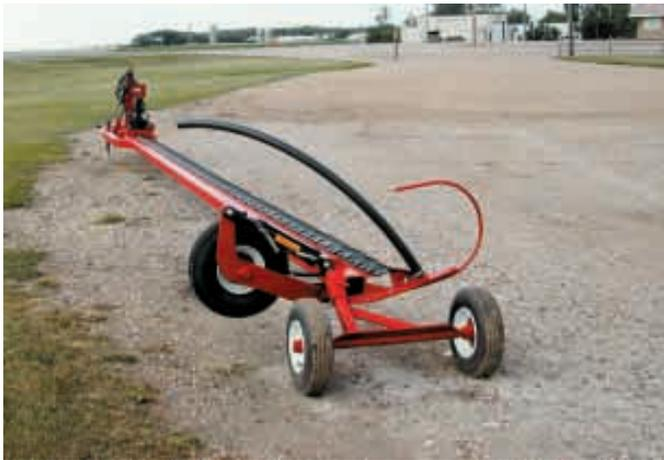
Faul's new 3-pt. mounted CRP Clipper is equipped with a Schumacher Easy Cut hydraulic sickle drive with instant reverse to clear a choked sickle.
