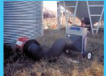
Hot water from furnace is plumbed into heat radiators that supply heat to bin-drying fans.
