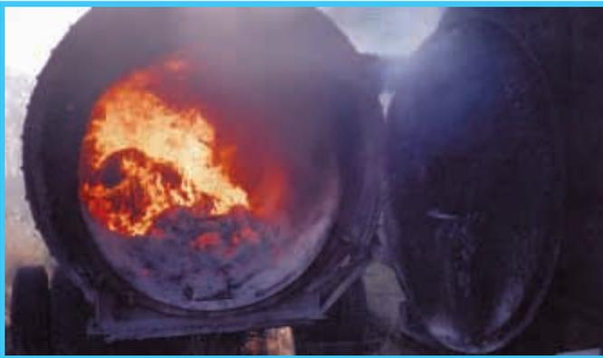
Heat from burning bales is used to dry grain and also to heat a pair of homes.
