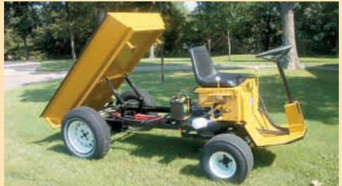
All models are equipped with hydraulic dump beds.
