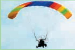
Prop is driven by a separate 100 hp engine that propels machine through the air at speeds up to 40 mph.
