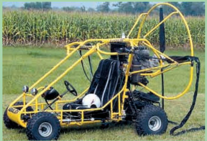
Powered parachute functions as an ATV when it's on the ground, powered by a 150 cc engine.
