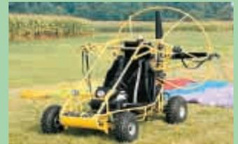
On the ground, machine is steered by a steering wheel. In the air, it's controlled by hand levers.
