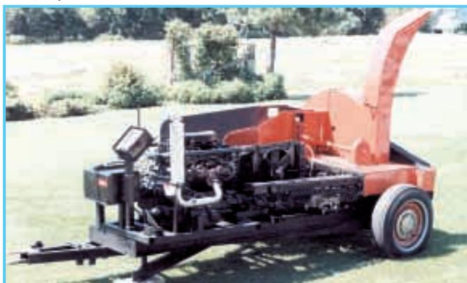
Trevor Shute converted an old 1-row, pto-driven hay chopper into this heavy duty brush chipper. Machine is powered by a 2.8-liter gas engine and 5-speed transmission.
