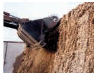
Bucket is tipped down to loosen the silage, then rotated back up to scoop up silage so it can be loaded into his TMR mixer wagon.
