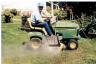
To clean the deck on his riding mower, Bernard Larson buries a length of garden hose under the lawn and runs it over to a spike-type sprinkler head that's buried in the ground.
