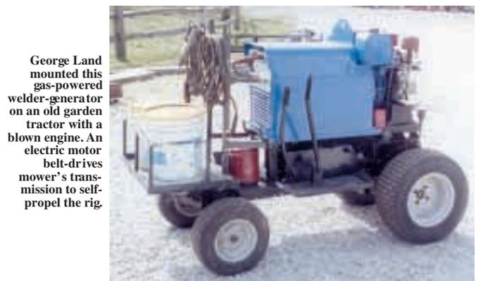
George Land mounted this gas-powered welder-generator on an old garden tractor with a blown engine. An electric motor belt-drives mower's transmission to self-propel the rig.
