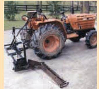
T.E. Salsman converted a 43-in. sicklebar and gearbox from an older walking mower to mount on his Kubota tractor. Gearbox is chain-driven by a hydraulic motor.
