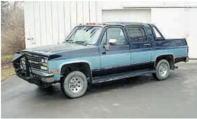
Weisbrod made a short box pickup out of this Suburban by cutting off the back half of the roof behind the second seat. Note home-built 3-pt. hitch and pto on front.
