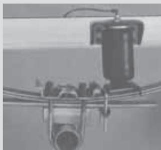
Air Lift helper springs add up to 2,000 lbs. of load-leveling support.
