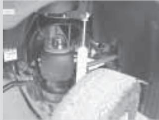
Kelderman's front lift kit for 2003 Dodge Ram pickups replaces factory coils with a large, high capacity air bag.
