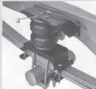
Firestone uses double-convoluted air springs for increased load-leveling and carrying capacities.
