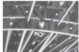
An extra set of holes makes it easy to shift tines when the other holes get worn.
