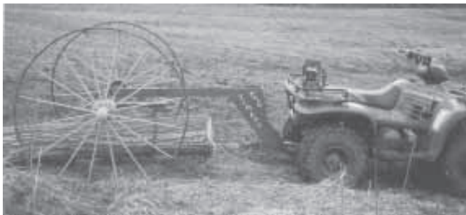
Rake is reinforced with braces and channel iron to make inexpensive log hauler
