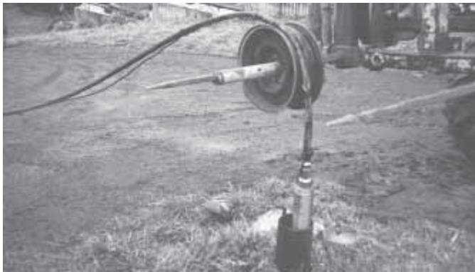
Old car wheel rim pulls long lengths of hose out of the well without kinking.
