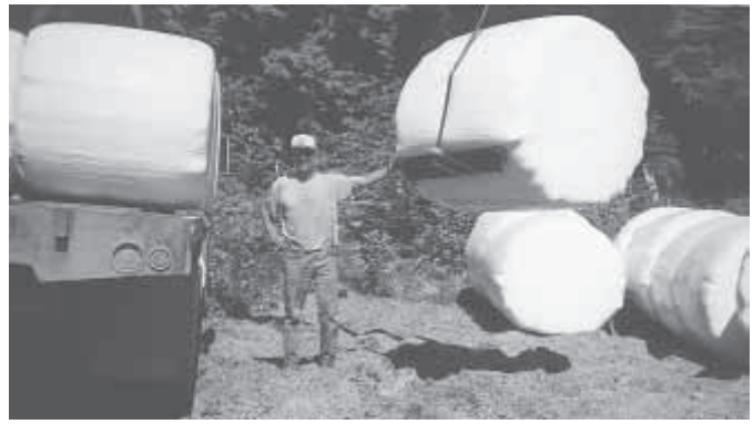
Modified tongs don't puncture or rip plastic-wrapped silage bales.
