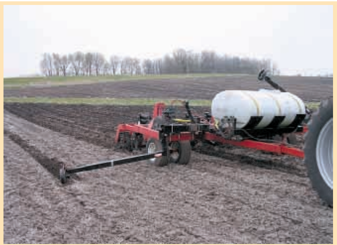
Manthey says the Zone Tool is especially effective in the spring, accomplishing in one pass what a disk or field cultivator did in two or three passes.
