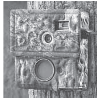
"PhotoHunter" is an infrared 35 mm camera that senses an animal and then automatically takes a photo of it.
