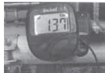
Sprayer speed - shown in tenths of a mile per hour - is displayed on a digital monitor on the operator's console.
