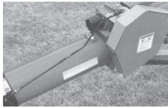
Gearbox resembles a small transmission, with a shifter that changes it from forward to neutral to reverse. Linkage and lever allows it to be shifted even when auger is raised and gearbox is too high to reach easily.
