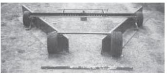
Harley Windrower can be mounted under any tractor or used as a pull-type to clear 8 to 10-ft. swaths of ground at a time.
