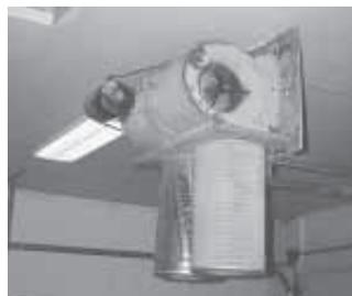
**Ben Kambeitz, Box 23027, Medicine Hat, Alberta, Canada T1B 4C7:** "By making use of an old furnace fan and a pair of used tractor air filters, I was able to come up with a low-cost air cleaner for my shop. It's a low-cost method of removing particles from the air inside a closed shop. The assembly
