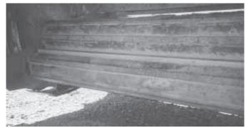
Chris Elliott, 4404 Breezy Point Road, McConnellsburg, Penn. 17233: "The rubber on the rolls on our Deere 1460 disc mower was coming off, which caused the machine to plug up. After pricing new rolls, we decided to fix the problem on our own. We stripped the rest of the rubber of f and welded six 1 1/2-in solid steel bars onto each roll
