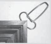
Spring-loaded clamps have sharp points that grip the wood firmly without cutting wood fibers.
