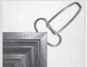
**Spring-loaded clamps have sharp points that grip the wood firmly without cutting wood fibers.**
