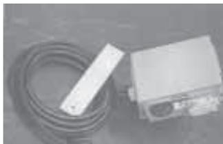
"Dump position locator" consists of a weather-tight box that encloses a red photo eye. Locator should be placed on a post or wall 3 ft. beyond pit or auger opening.
