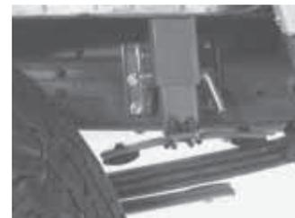
When you expect to do some heavy hauling, just lower the arm and secure it in place with a lynch pin.
