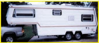
I built this 24-ft. long fifth wheel camper back in 1979, when there weren't any like this on the market yet. I used light gauge, 1 1/4-in. rectangular tubing to build the frame and mounted it on the chassis of a Dodge pickup. I installed the tubing every 16 in. on the floor and ceiling and pop riveted an aluminum skin to it using aluminum roofing sold by Sears.
