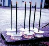
I came up with low-cost portable posts by anchoring steel fence posts in car wheel rims filled with concrete. The rims can easily be rolled to nearby locations. They come in handy whenever I take my collection of antique tractors to shows. By tieing yellow rope between the posts I can quickly rope off my tractors. (Don Peck, 212 No. Elm St., Zearing, Iowa 50278 ph 641 487-7306)
