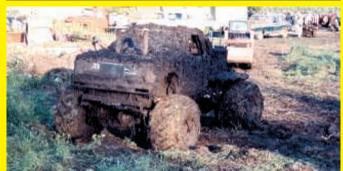
My home-built, 4-WD, articulated "mud truck" can get in and out of just about any mud hole and works great for hill climbing. It's fun to drive. I built it by modifying a junked-out 1978 Chevrolet 1-ton pickup.
