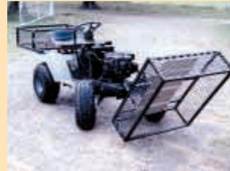
Machine has two large expanded metal baskets. The one on front tilts forward for access to engine.
