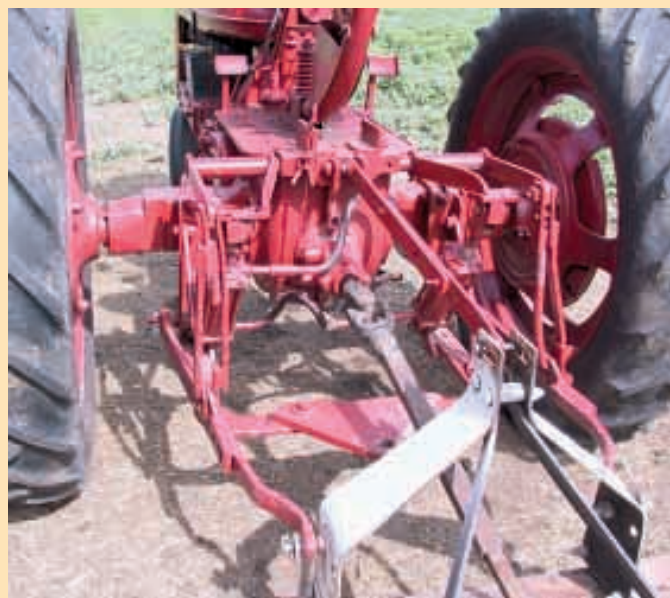
"I built the whole thing with scrap I had laying around, except for some pins for the ball joints," says Larry Francis about the 3-pt. hitch he added to his Farmall H.
