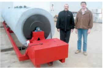
Biovator is a mechanical composter that mixes carcasses with wood chips inside a revolving insulated tube. It's turned by a 1 hp motor.
