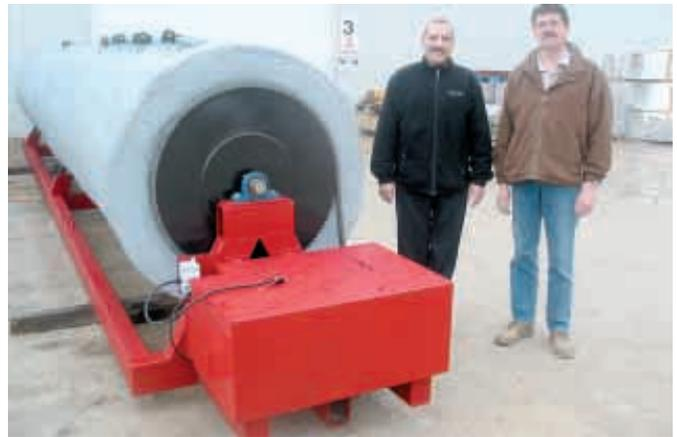
Biovator is a mechanical composter that mixes carcasses with wood chips inside a revolving insulated tube. It's turned by a 1 hp motor.
