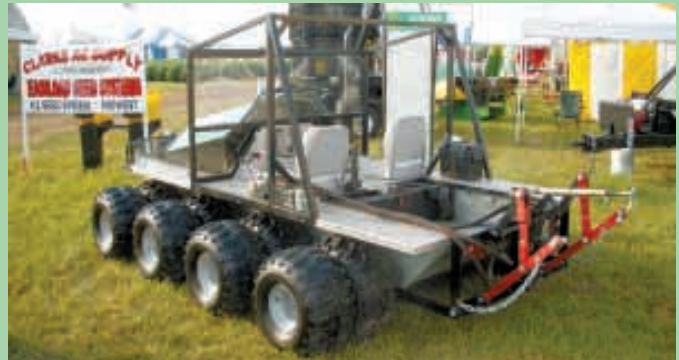
Built from off-the-shelf parts, the all-wheel drive is designed for easy maintenance.
