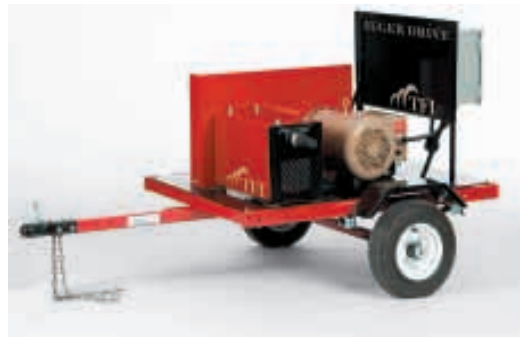
Built from off-the-shelf parts, the all-wheel drive is designed for easy maintenance.
