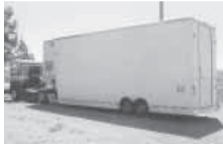
Portable slaughter house has an interior height of 10 ft. 6 in. Cattle are skinned and gutted inside but cutting and wrapping are done elsewhere.
