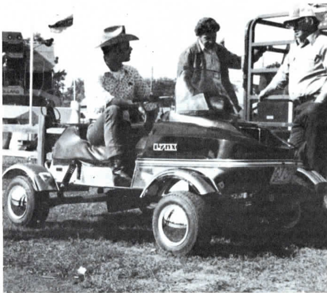
Harold Parrow's new Mini-Wheel kit adapts to 11 makes and models. Top speed is about 20% faster than machine will go as a conventional snowmobile running on snow. Takes about 3 hrs. to install.
