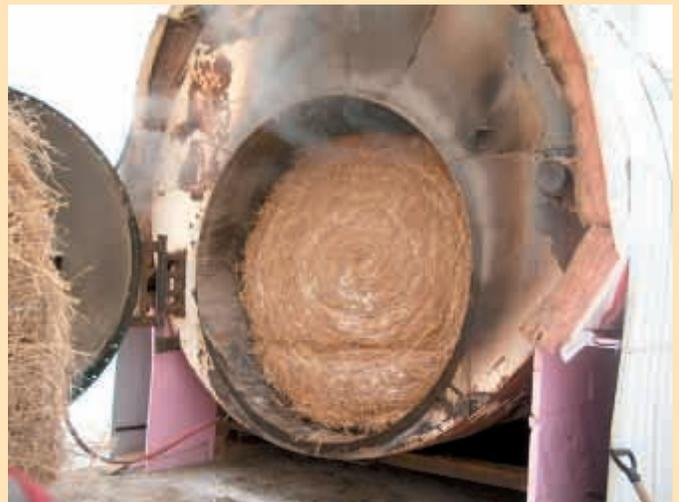
Up to three 5 by 6-ft. round bales can be loaded into furnace at one time.
