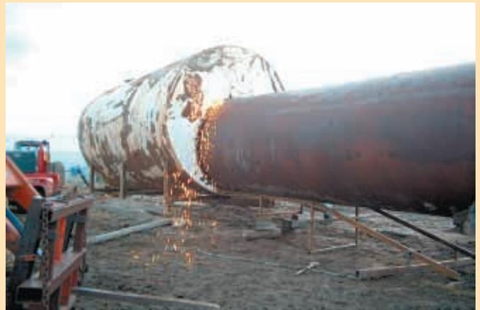
Giant firebox was made by inserting a 7-ft. dia. underground fuel tank into a larger 11-ft. dia. tank.
