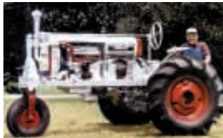
Special Farmall prototype 1927 Regular has a single front wheel.
