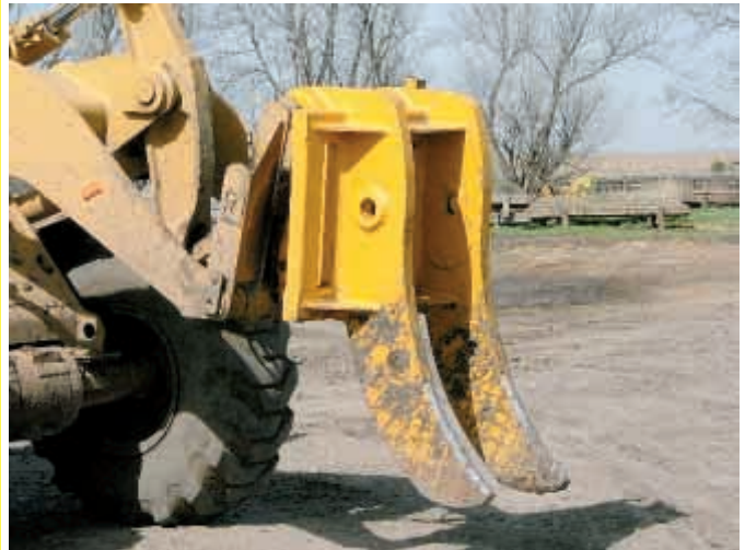
Rock digger mounts on Rausch's Cat Payloader. Its two 6-ft. long teeth can penetrate the ground to a depth of 2 ft. and dig out rocks up to 6 ft. in diameter or even bigger.
