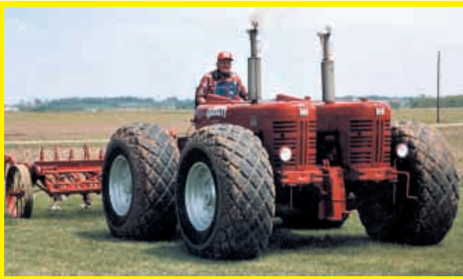
Harry Lee's "newest" tractor is a 1956 factory-built prototype from Garrett Mfg. It's called the Twin Drive 400 IHC diesel.
