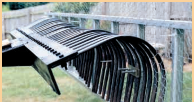
Ladder bolts onto rake tines. Chicken wire is tied to it with wire.
