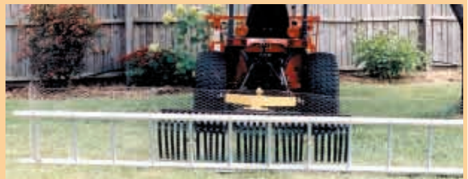
Jay Main rakes leaves with a 16-ft. wide section of aluminum ladder. It's covered with chicken wire and hooked on behind his 3-pt. mounted landscape rake.
