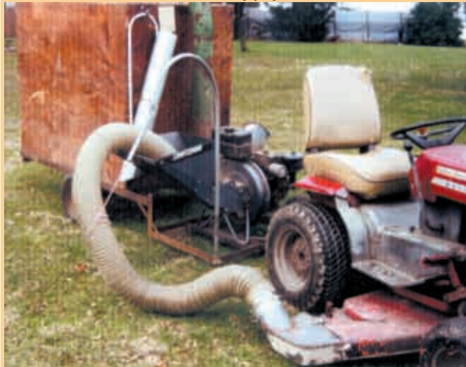
Gas-powered shredder not only picks leaves up, it also shreds them on-the-go. Unit blows leaf bits through a dust collector and then into cargo box.
