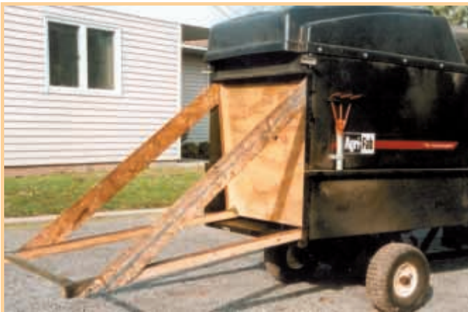
Slide-out unloader pulls entire load out of Johnson's Agri-Fab blower vac.
