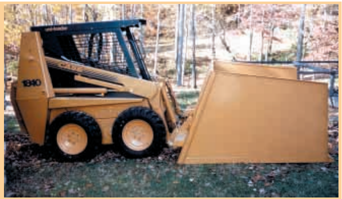
Skid steer loader-mounted “leaf bucket” is made from light gauge sheet metal. Matthews simply rakes or scoops leaves into bucket.
