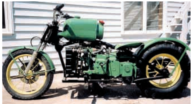
Pat Prom’s home-built Deere motorcycle has big implement-style wheels with spokes.
