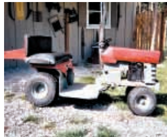
When Bill Wilson converted a garden tractor to run on electric power, he made his own electric motor.
