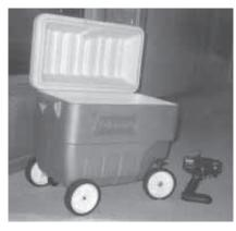
Cooler is equipped with a DC gear motor and steering system and operated by a remote control transmitter.
