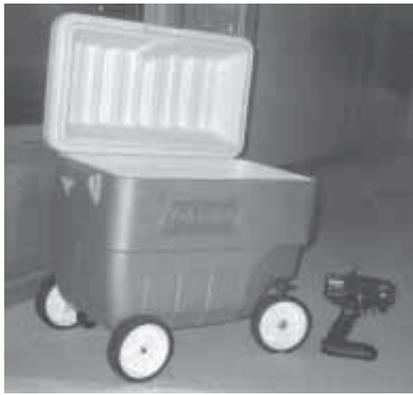
Cooler is equipped with a DC gear motor and steering system and operated by a remote control transmitter.
