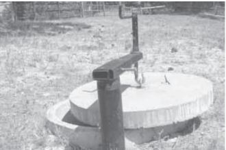
Horizontal bar with a crank shaft on the end is used to lift cover off septic tank. Crank-Style "Cover Remover"
