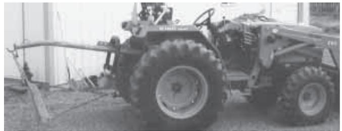
Rail hangs from 3-pt. mounted posthole auger frame so it's easy to get into corners.
