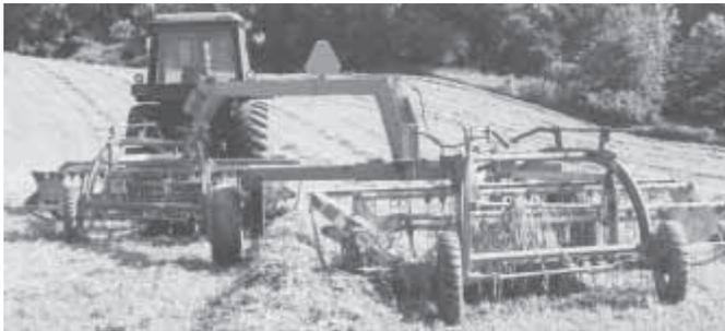
A lengthened Hesston 1024 hydra swing frame pulls a left and right hand rake at the same time.
