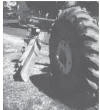
Robert Rodenberg tips blade to steepest angle and drops front end into ground about 2 ft. from post. Before blade gets to post, he raises it to pull post out.
