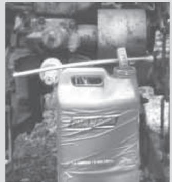
A 16-in. long plastic toilet supply line, inserted through lid, serves as spout to pour chemical into oiler.
